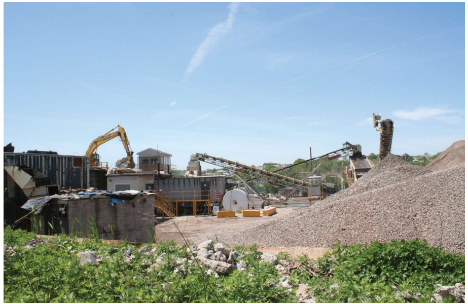
Turning C&D waste into aggregate for future construction, Town of Kearny, NJ. Photo © Erik Kiviat
